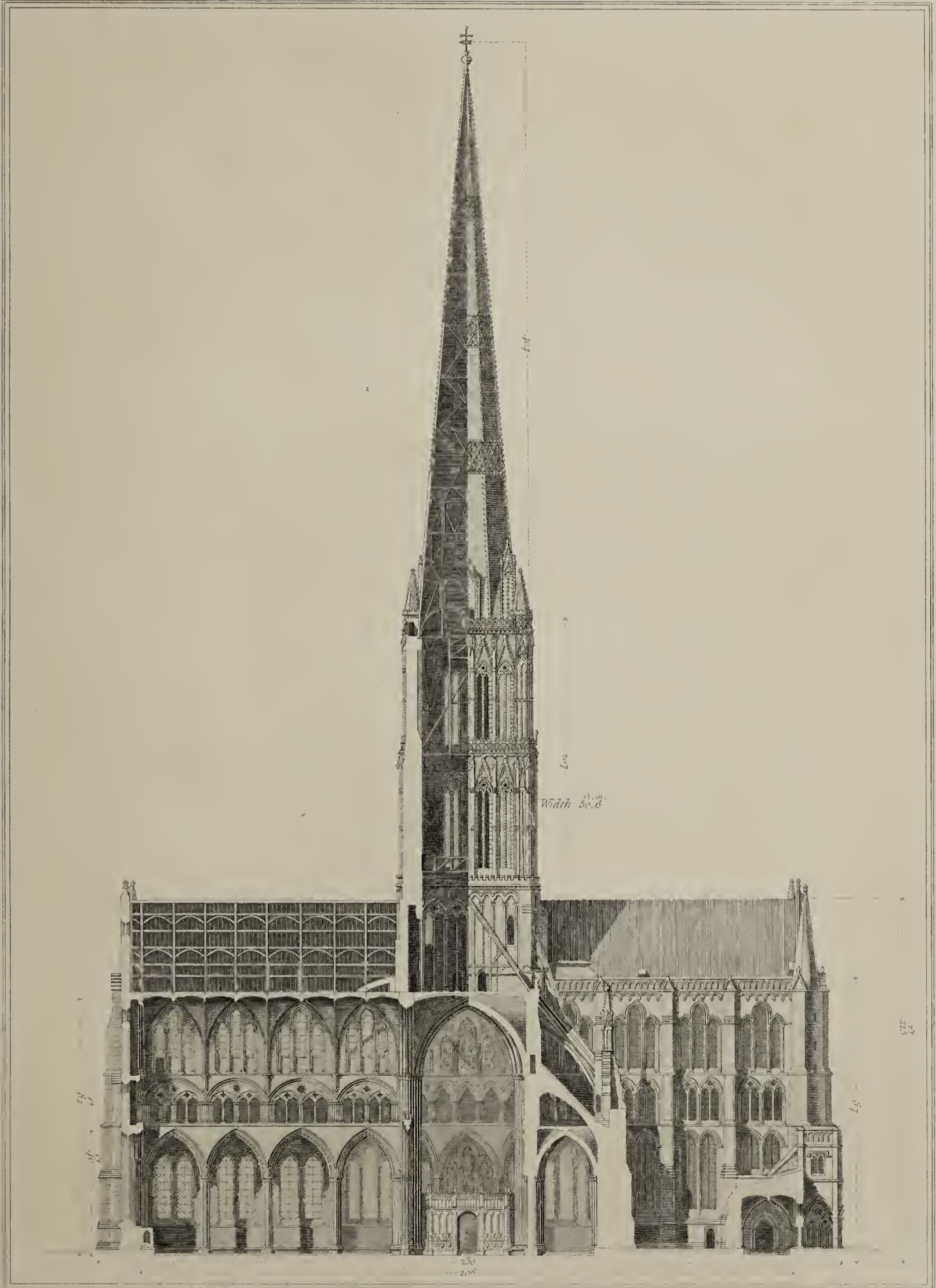
Drawn by R. Cattmole. Engraved by G. Charlwin. for Britton's History &c. of Salisbury Cathedral SALISBURY CATHEDRAL Section & Elevation of the great Transept, Tower & Spire. London: Published April, 1836, Longman & Co. & Waterhouse Rev.
